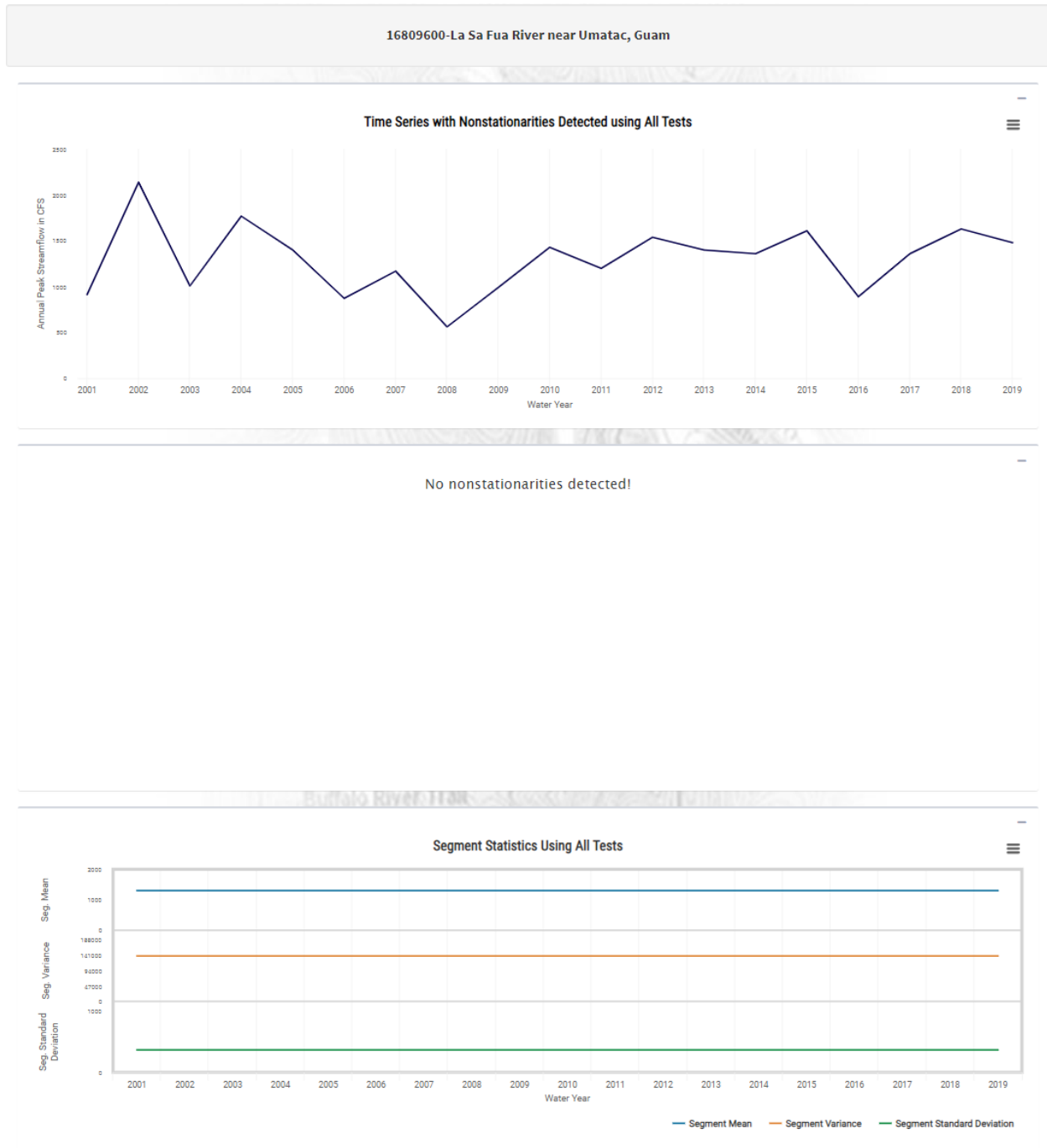
Plate 1. Nonstationarity Analysis of Maximum Annual Flow, La Sa Fua River near Umatac, Guam (2001-2019)
